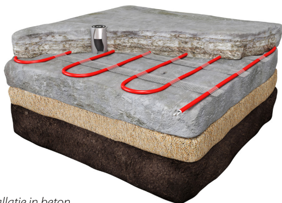
Installatie in beton
