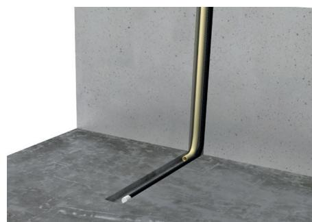
**TAKE CARE:** Never place the sensor in the vicinity of a (hidden) radiator pipe! Never install it passing under a heating cable!
