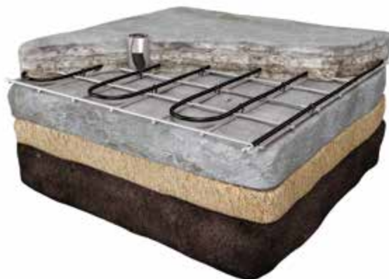
Installatie in beton
